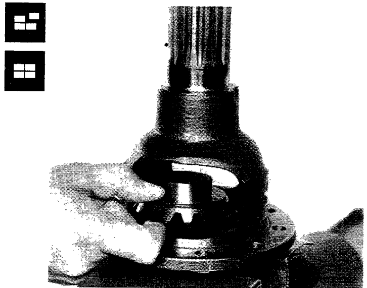
Removing-refitting planet wheels from differential casing
